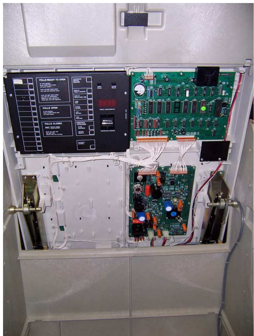
Under the back panel: officer's control panel (left), micro – controller (top-right) and power supply controller (bottom-right)
