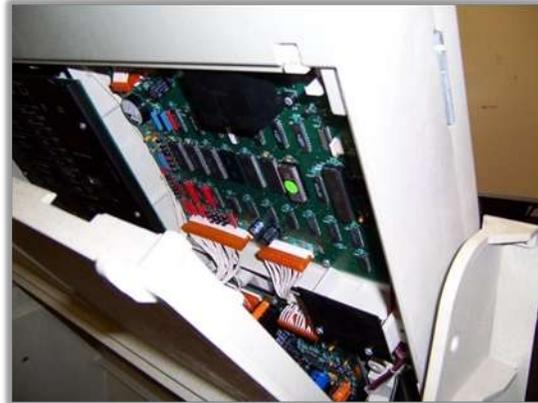
*Figure 2: Service Panel Exposing Motherboard*
